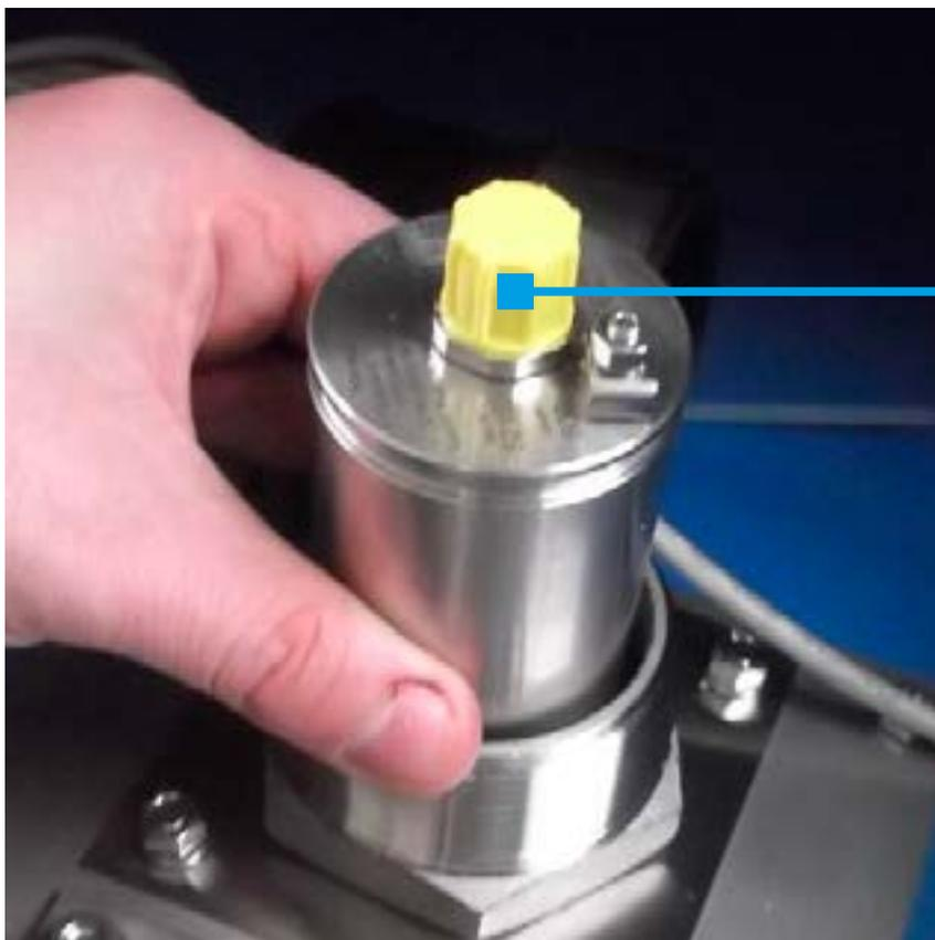
**SONDA DI MISURA LIVELLO
